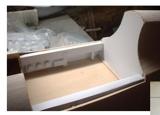
The cockpit is an area where I chose to compromise scale appearance for airframe integrity. The **Ziroli** fuselage is built on a 1/2" x 1/4" spruce crutch inside formers. The crutch is stiffened with 1/2" x 1/8" spruce diagonal bracing between the formers. The cockpit area is directly above the open wing mount
