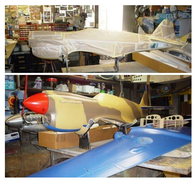
And now the last colour to be applied is the cockpit green to the wheel wells as per the picture of the full size below.
