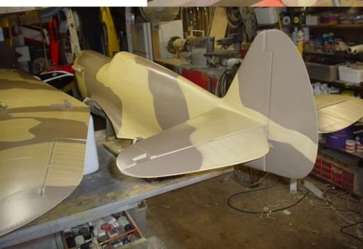
Masking removed. Next step is to fully mask the upper surfaces of fuselage and wing and paint the underside with the very different Dark Mediterranean Blue that Ross has used on his P40.
