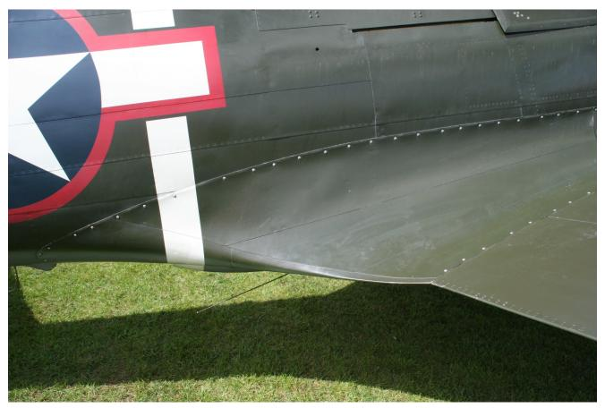
The root fairings on the wing, tailplane and fin are all fastened to the airframe with machine screws, I fudge these by applying the usual dabs of PVA and when dry, carefully sand the domed tops on the glue blobs down to be nearly flush with the surface.
