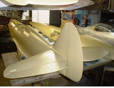
rear glazing and canopy. I will follow all of that up with another coat of Mid Stone and then a coat of the Dark Earth camouflage before masking the complete top surfaces of the plane and attacking the underside.
