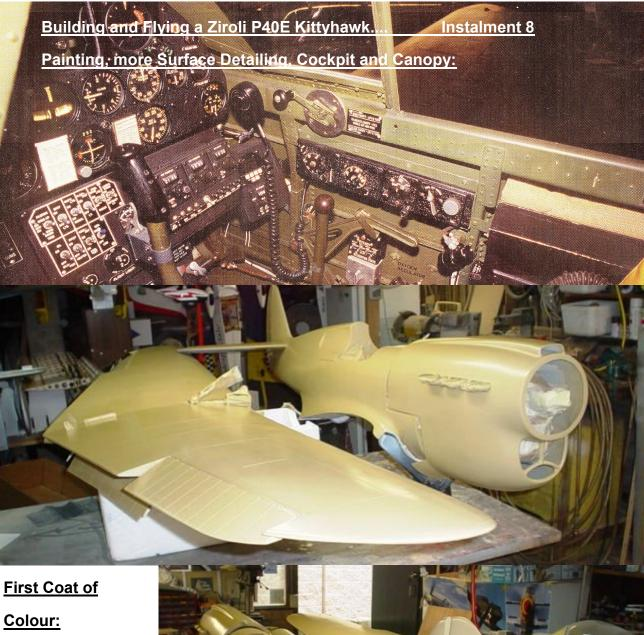
After removing all the panel line tape the plane was sprayed with the first coat of the Mid Stone colour.
