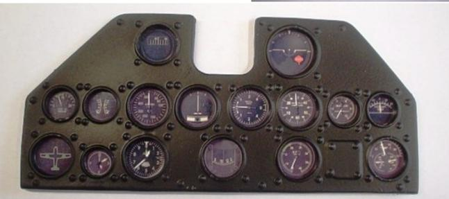
The instrument panel is a major feature and is made up in four layers, a backing sheet of PVC, a printed instrument sheet over, a piece of clear PVC over that and finally the pre painted vac formed panel on top. Sounds fiddly but is easy to do with the **DB** kit of parts.
