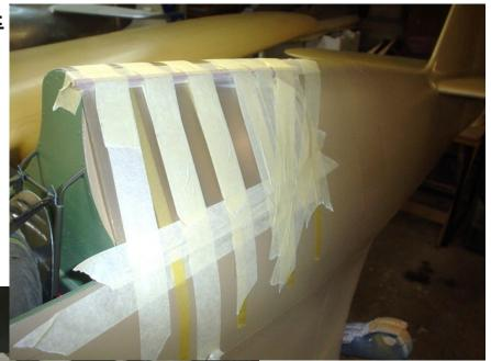
with ZAP canopy glue. The canopy was then masked up with the good Tamiya stuff, edges roughened up with sandpaper and it was then glued over the side windows to the fuselage and strapped down with a fair bit of masking tape.
